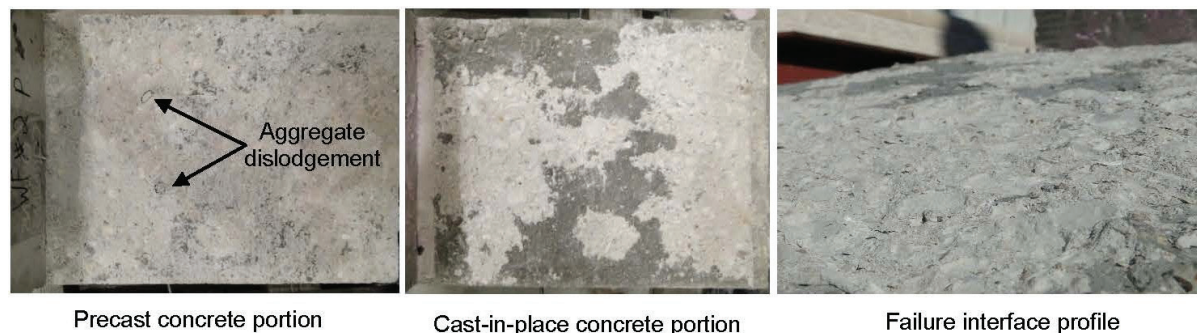
Figure 18. Wood-float-finished specimen L-WF-2 at failure.
