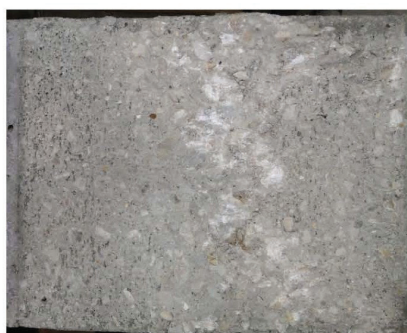
Typical CSP 7 specimen failure interface profile
