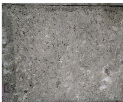
Typical CSP 8 specimen failure interface profile
