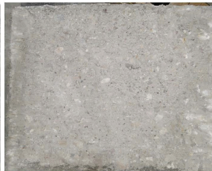
Typical CSP 6 specimen failure interface profile
