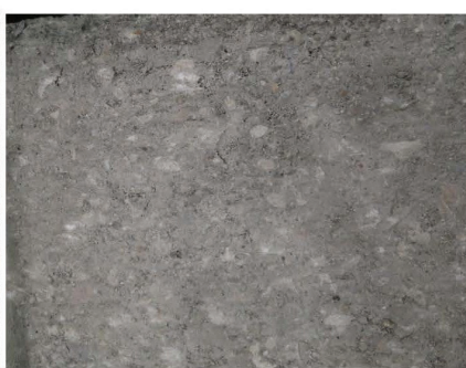
Typical CSP 9 specimen failure interface profile
