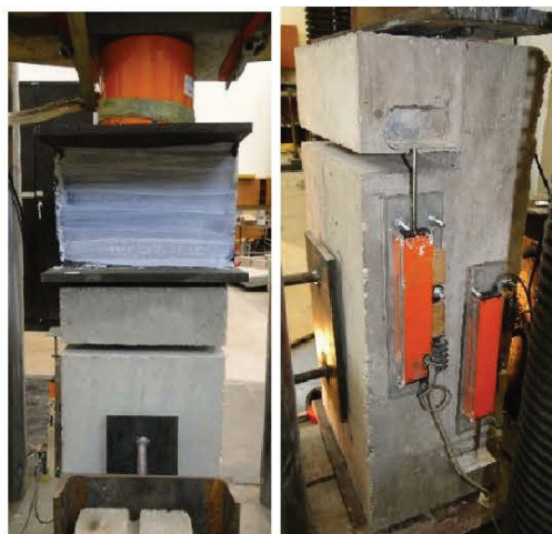
Figure 14. Test setup for push-off tests evaluating the cohesion factor. Note: CIP = cast-in-place concrete; LVDT = linear variable differential transformer. W12 × 79 = W310 × 118; 1" = 1 in. = 25.4 mm; 1 kip = 4.448 kN.
